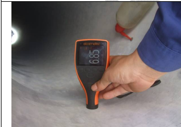
Cement lining thickness
