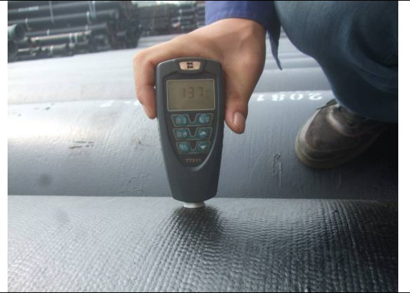
Bitumen coating thickness
