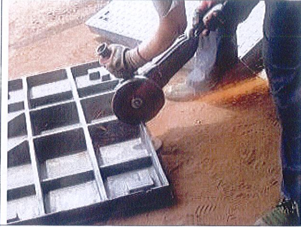
Taking sample for chemical analysis
