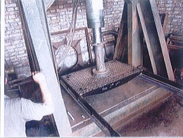
2/3 load test for permanent set
