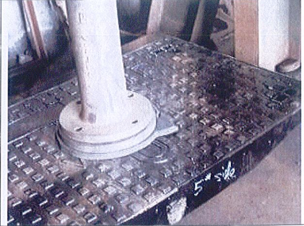
2/3 load test for permanent set
